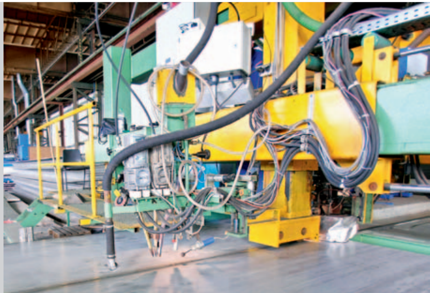
Welding of the first seam to form a plate with the required width
