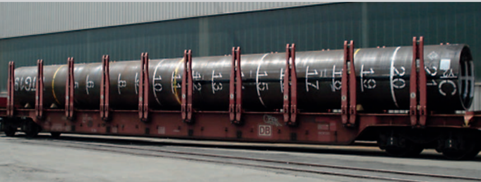
LWDS Pile OD 1828 x 50 x 25000 mm (72" x 2" x 75,5') complete with internal grouting beads ready for shipment
